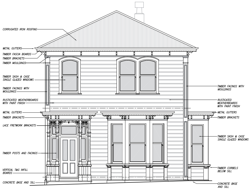
PIPITEA STREET ELEVATION (NORTH)
