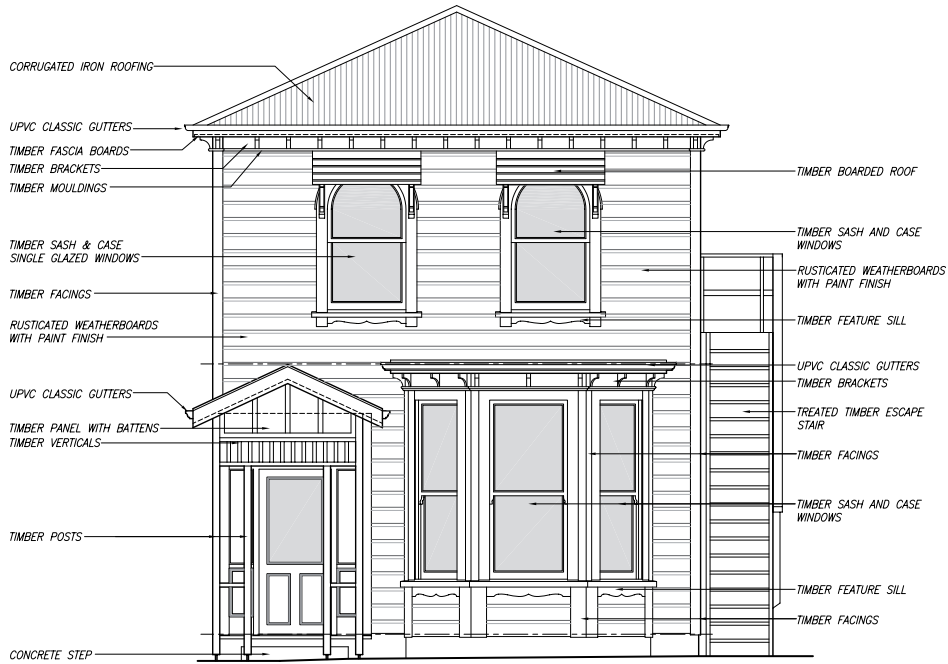
PIPITEA STREET ELEVATION (NORTH)
