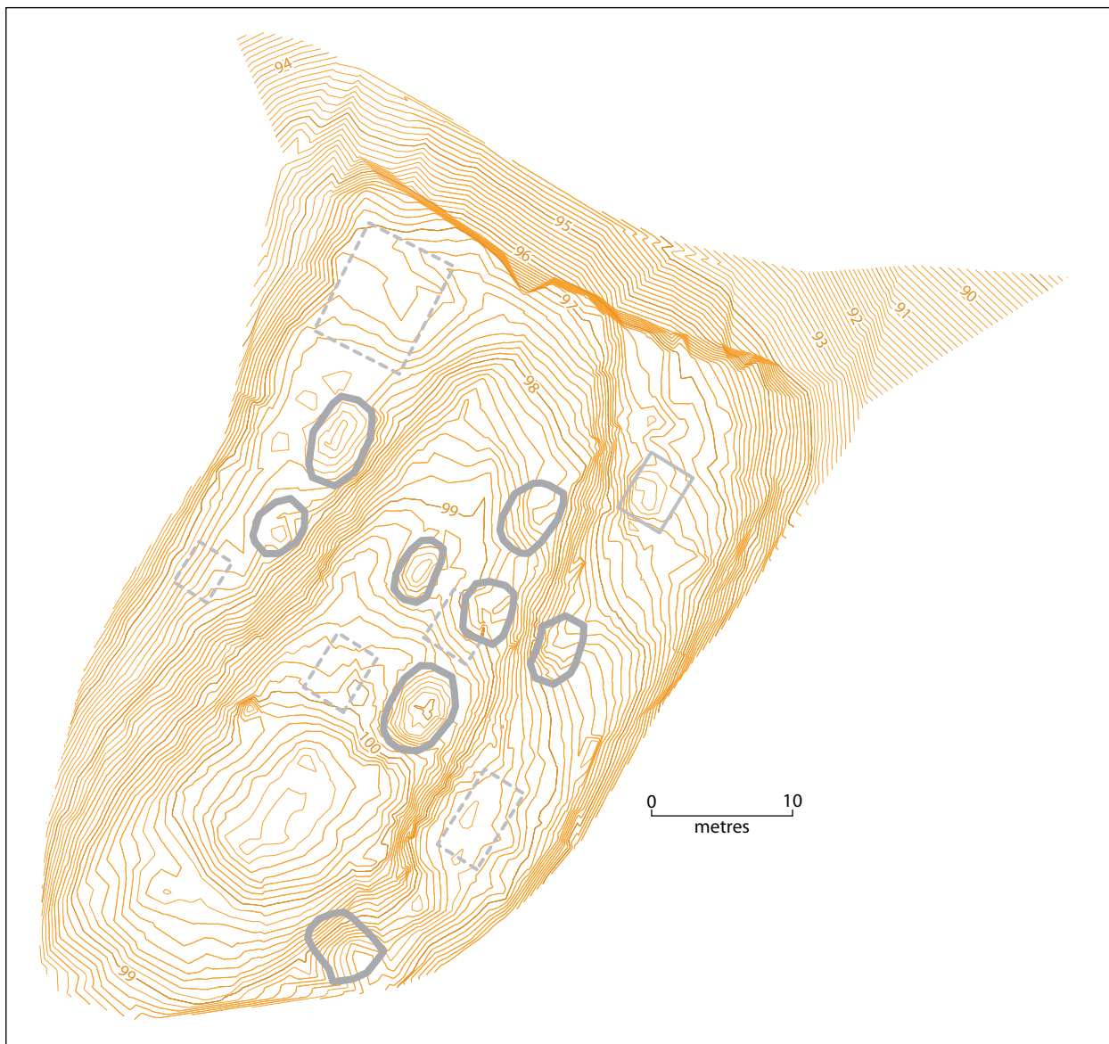
2. Topographic map of pa P04/640. The pits visible on the ground are outlined in heavy grey, pits visible in 2003 are sketched in with indistinct pits shown in a dashed line. Contour interval = 10 cm, major contours = 1 m.
